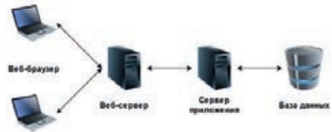
Figure 3. Layered web application architecture
