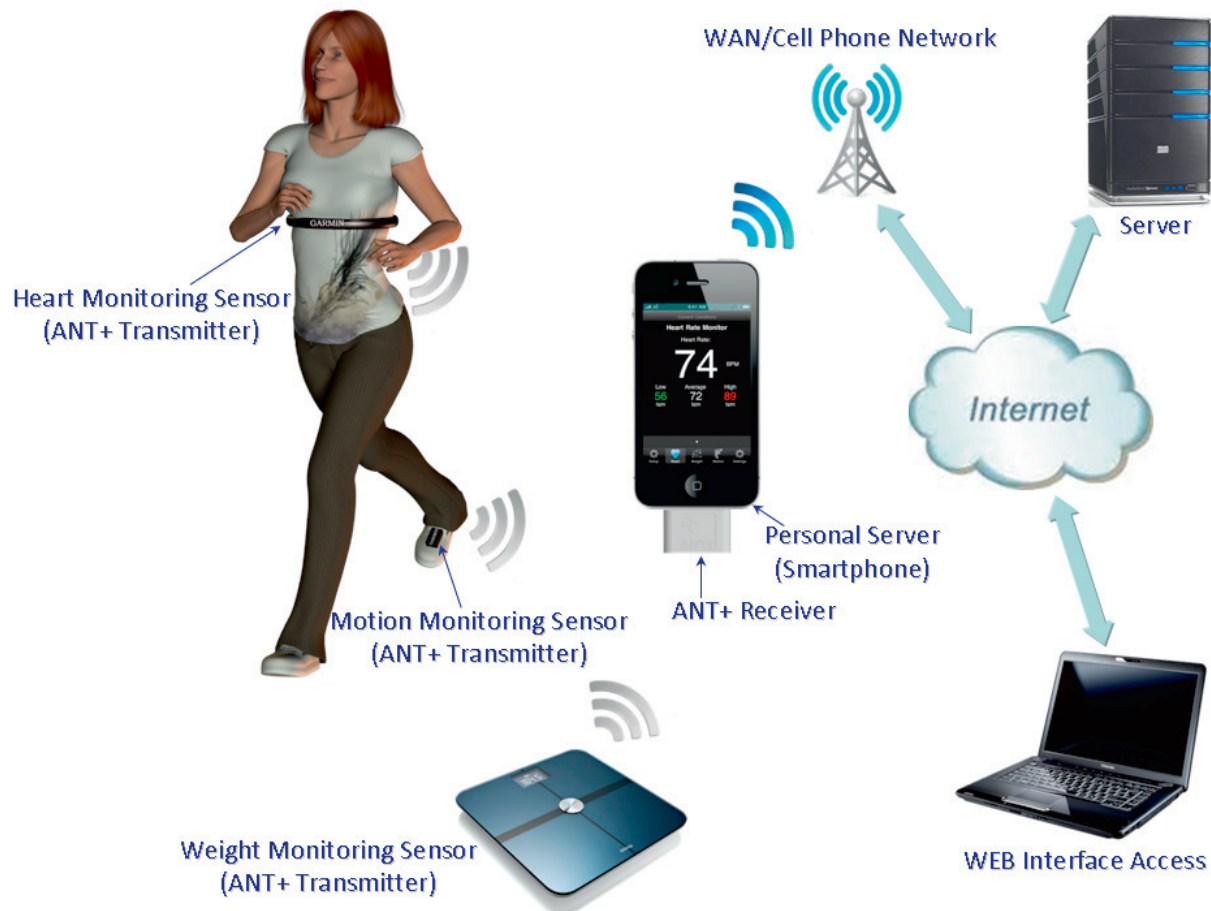
FIGURE 3. SYSTEM ARCHITECTURE OF THE UAHEALTH
