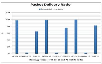
Figure 4. Comparison of PDR for AODV, DSDV and DSR for 15, 35 and 75 nodes
