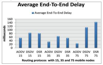
Figure 5. Comparison of AEED for AODV, DSDV and DSR for 15, 35 and 75 nodes
