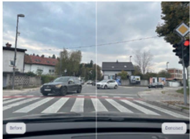
Figure 4. Result of noise removal from the image
