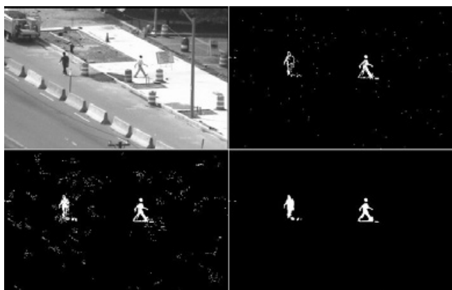
Figure 3. Background subtraction. Source: http://vip.bu.edu/projects/vsns/background-subtraction/fa/ .
