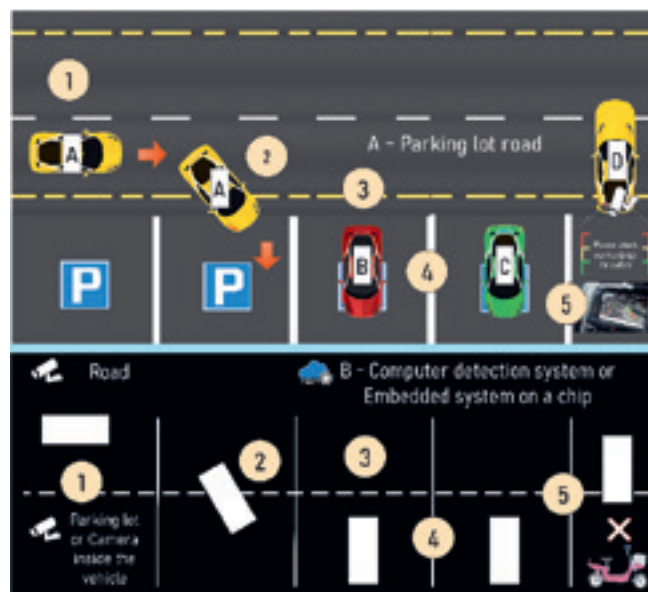
Figure 5. Working idea proposal for the Method in detection of parking occupancy on chip (ComDPOCh). Source: author's contribution.
