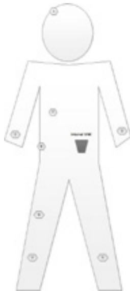
Figure 1. WBAN network, arrangement of nodes on the body used for simulation
