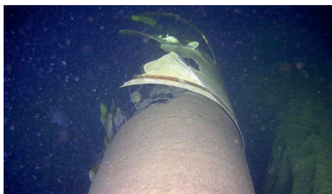
Fig. 3. The damaged offshore Balticconnector gas pipeline. Source: [8]
