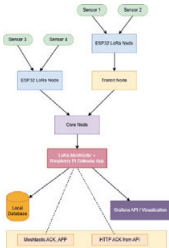
Figure 2. LoRa Meshtastic Gateway System – Data Flow Diagram and Acknowledgment Structure
