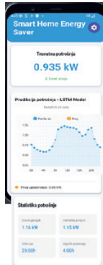
Figure 3. Main interface of the Smart Home Energy Saver application displaying real-time electricity consumption, 24-hour LSTM-based forecasts and peak consumption statistics for proactive energy monitoring.
