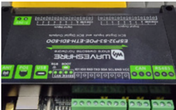
Figure 5. Hardware platform of the main ESP32-S3 control node with CAN and RS485 interfaces
